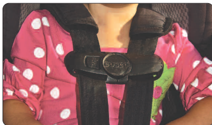
Plastic harness retainer clip should be at child's armpit level.
