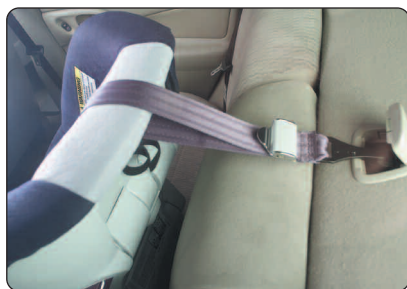
An anchor option for tether hook
