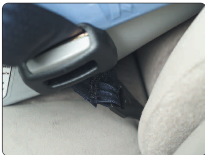
Flexible LATCH hook using anchor bar
