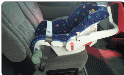
Rolled towel for angle when using seat without the base.
